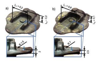
Fig. 2. The view of the forgings after the forging process: a) initial forging phase – unworn tools, b) final forging phase (worn die inserts) – enlarged dimensions of the tool and the forging
